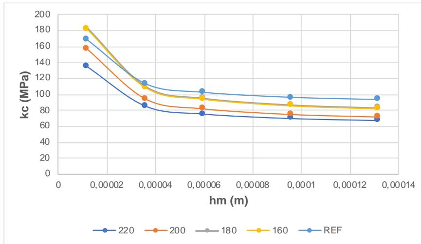
**Figure 2.** Dependence of specific cutting resistance on uncut chip thickness
