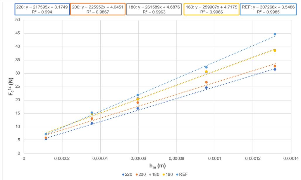
**Figure 1.** Dependence of cutting force per one tooth on uncut chip thickness
